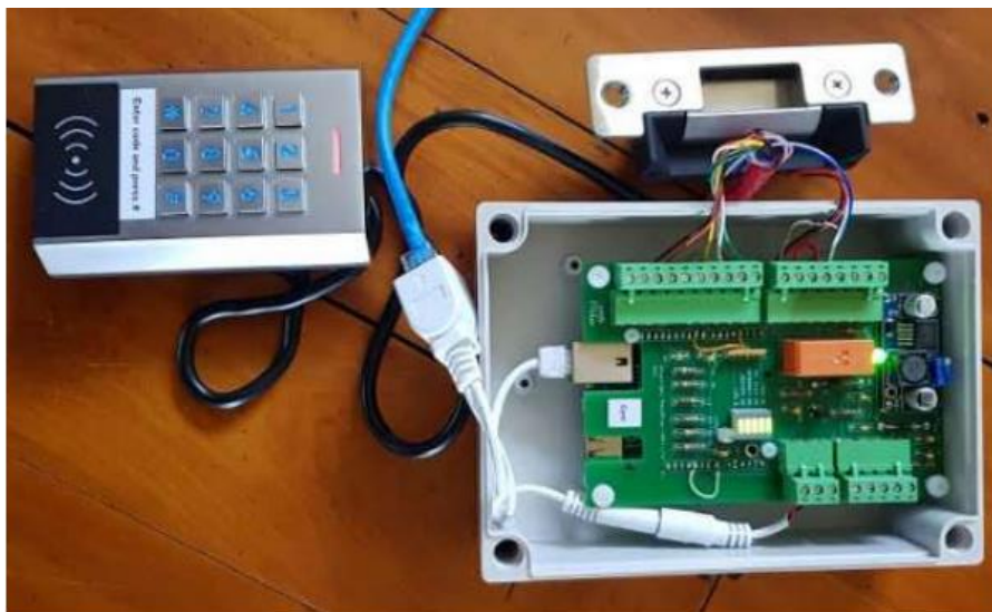
Figure 1: The door controller in a separate box with peripherals connected under test and POE.
